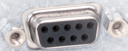
RS232 standard on all General Protocol, Advanced Protocol and Advanced Protocol Security models/sizes
